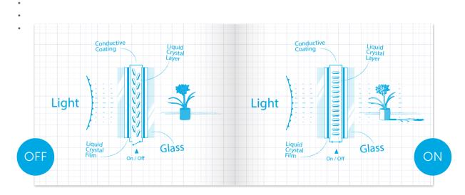
Randomly aligned LC molecules scatter the light, making the glass opaque, ideal for projection, privacy, and drawing. Electricity from Gauzy controller arranges the LC molecules on demand, making the glass transparent, for an open clean atmosphere.
