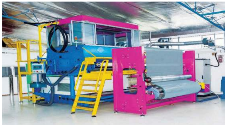
Figure 1. Gauzy roll-to-roll PDLC film manufacturing line.
