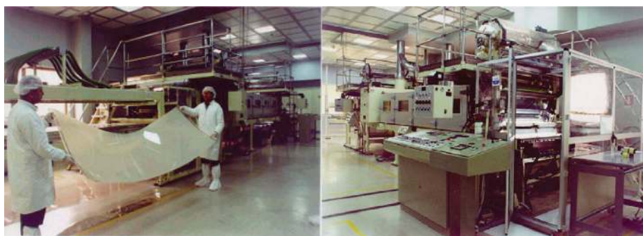
Figure 2. Snia's first multifunctional PDLC film pilot plant.
