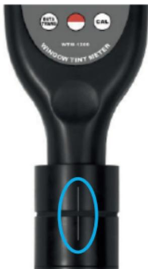
4.3 Connect the two sides of the probe of the Tint meter to each other. Make sure the markings on the probe are aligned with each other.
