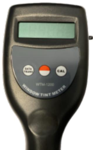
4.2 Turn on the Tint Meter by pressing the middle button marked with a half-filled circle.
