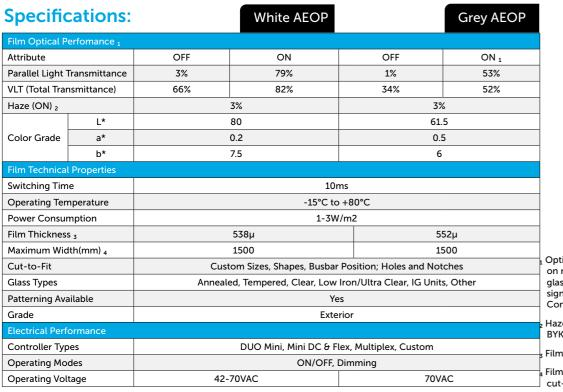
Optical Performance measured on retrofitted film on clear glass at 25°C using square wave signals provided by Gauzy PDLC Controllers, at 70 VAC
